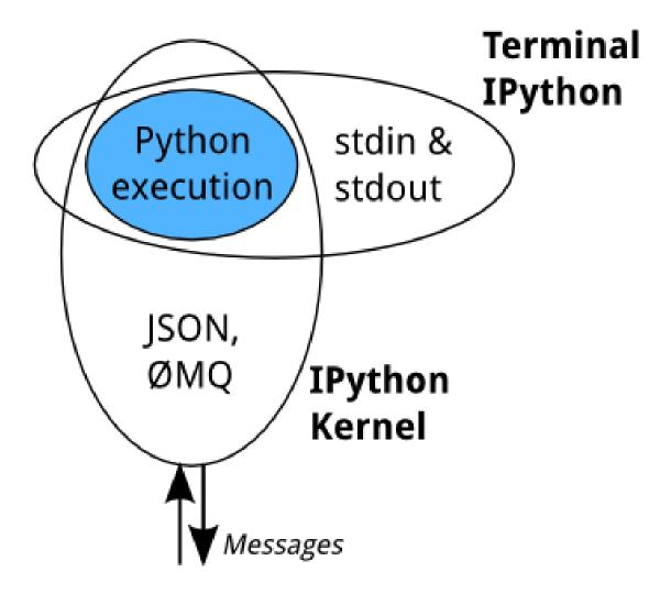
A kernel process can be connected to more than one frontend simultaneously. In this case, the different frontends will have access to the same variables.
